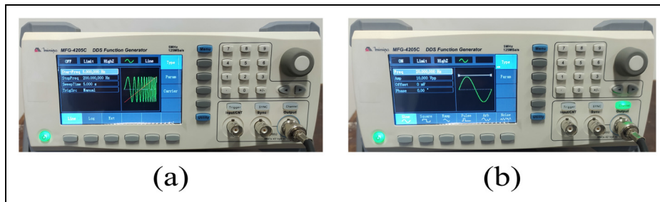
Figure 11. Visualisation of the signals in the frequency generator that will be mechanically replicated by the shaker: (a) Sweep signal and (b) constant-frequency sinusoidal signal.
