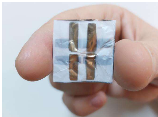
Fig. 6: Photograph of a selected sample of a complete fabricated device, already with the electrical contacts deposited on both sides of the BNC.
