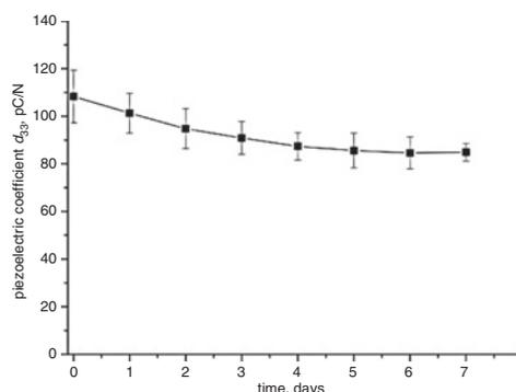
**Fig. 2** Piezoelectric coefficient  $d_{33}$  plotted against time, indicating decay of 18% of its initial value
