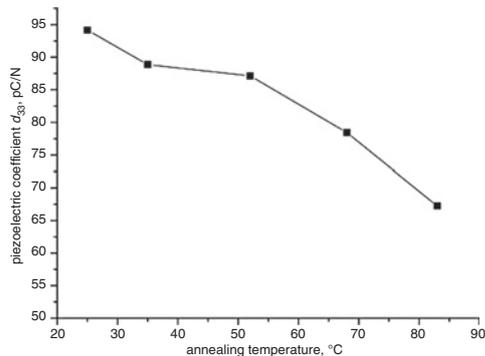
**Fig. 3** Piezoelectric coefficient  $d_{33}$  after exposing piezoelectrets for one hour at specific temperatures
