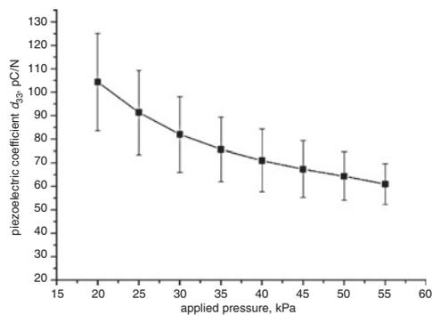
**Fig. 4** Influence of pressure on piezoelectric coefficient  $d_{33}$  of 3D printed ABS piezoelectrets
