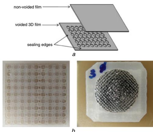
**Fig. 1** Concept of piezoelectret 3D printer sensor before assembling films (Fig. 1a), and top view of 3D printed voided structure and piezoelectret sample with electrode (Fig. 1b)
