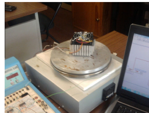
Fig. 2. The measurement setup showing a thermoelectric modules model TEC1-12707 between a controlled hot-plate and a controlled cooling fan. The personal computer running the LabView software connects to a data acquisition board model NI USB-6009 for controlling the heat flow (by way of the controlled hot-plate and the cooling fan) and for measure the produced currents and the respective voltages.
