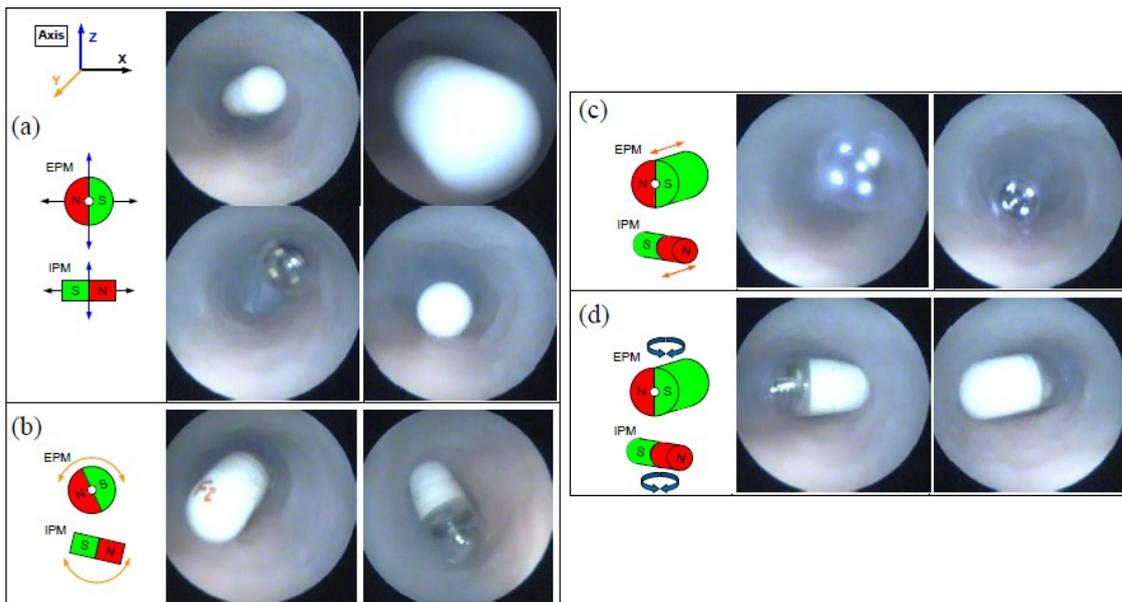
Fig. 3. EC movements when actuated by the EPM; (a) Forward and backward, lifted and lowered; (b) Tilt up and down; (c) Left and right translation; (d) Tilt left and right.
