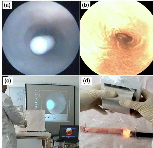
Fig. 4. Clinical tests in porcine intestine; (a) Fiber colonoscope image; (b) EC image; (c) Remote control of the EC by a technician; (d) Manipulation in detail of the EPM.
