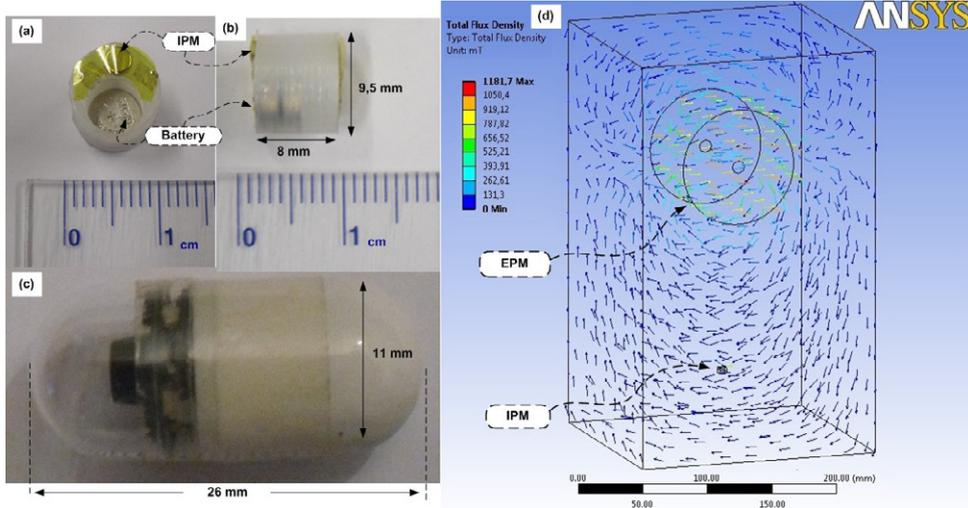
Fig. 2. IPM and battery inside of the EC (a) Topview; (b) Side view; (c) The modified EC (IPM and new battery inside) maintaining the standard size; (d) FEM simulations for study of the magnetic field between the EPM and IPM.
