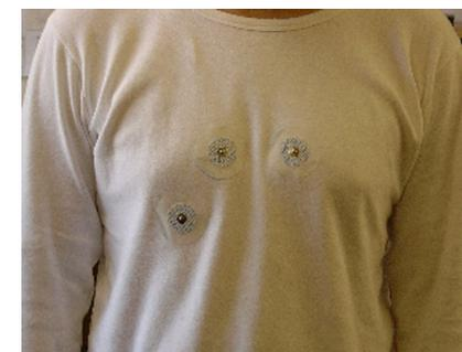
Fig. 8. A photo of the patient wearing a electronic shirt ready to plug the RF microsystem (antenna + transceiver). We can see the three connections for heart rate with a single electrode, respiratory function and posture.
