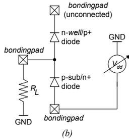
Figure 5: Used setup for obtaining the  $I/V$  characteristics of the (a) n-well/p+ and (b) p-substrate/n+.
