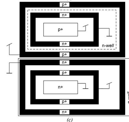
Figure 2: (a) Lateral projection of a CMOS inverter; (b) equivalent circuit due to the latch-up phenomena (Ker *et al* 2003b); and (c) used isolation technique for preventing latch-ups.
