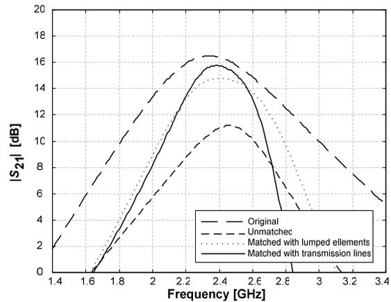
Figure 9: Simulated  $|S_{21}|$  [dB] of the LNA.
