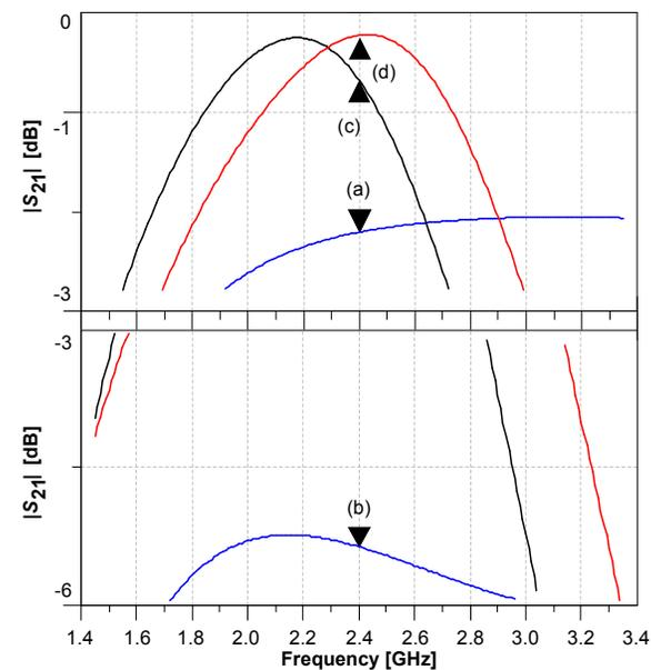
Figure 13: The  $S$  parameter measured from the output of PA to the input of antenna obtained (a) ideally, without the effect of the ESD protections; (b) with the effect of the ESD protections; (c) with compensation network formed by lumped elements; and (d) with a compensation network formed by transmission lines.
