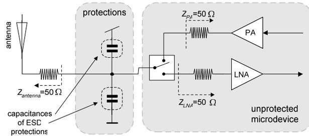
Figure 3: The possible effects that can result with the presence of ESD protections.
