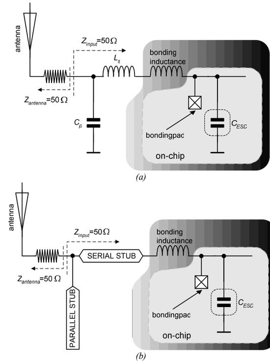
Figure 6: Matching networks for compensating the effects that arise due to the capacitances of the ESD protections for the following implementations: (a) with lumped circuit-elements, and (b) with transmission lines.
