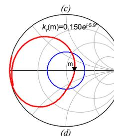
Figure 7: Simulations showing the reflection coefficient,  $k_R$ , at the input of the LNA obtained: (a) for an ideal situation without considering the effect of ESD protections; (b) for the unmatched situation, considering the effect of ESD protections; (c) for a matched situation, considering a compensation network made of lumped elements, and (d) for a matched situation with a compensation network, implemented by transmission lines.
