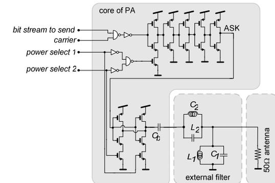
Figure 11: The schematic of the transmitter.
