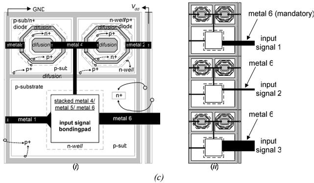
Figure 1: (a) The most common configurations for protecting against ESD discharge, when doing a design of a RF chip. (b) Chip layout and respective protections of the RF transceiver used as case study. (c) Schematic showing the construction details of a bondingpad for input signals protected by n-well/p+ and p-substrate/n+ diodes and connection with three bondingpads with ESD protections.
