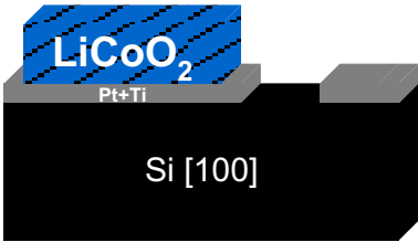
FIG. 40: DESIGN OF BATTERY CATHODE (THICKNESS WAS EXAGGERATED FOR BETTER VISUALIZATION).
