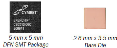
FIG. 4: THIN-FILM BATTERY CBC012 MARKETING BY CYMBET, AT RIGHT WITH ENCAPSULATION OF INTEGRATION WITH OTHER INTEGRATED CIRCUITS [14].
