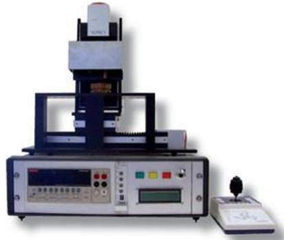
Fig. 52 – Scanning probe instrument for spatial resolution of the Seebeck coefficient and the electrical conductivity – SPM-Potential-Seebeck Microprobe (Courtesy of D. Platzek).
