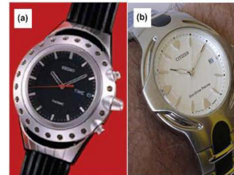
Fig. 5 - Thermoelectric wristwatches; (a) Seiko Thermic; (b) Citizen Eco-drive Thermo.
