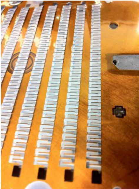
Fig. 48 – Developed thermoelectric devices in polyimide foil of 50  $\mu\text{m}$  of thickness.
