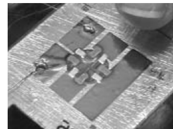
Figure 11: A photograph showing a thermoelectric converter made with four pairs of planar thermoelectric p- and n-type materials. The p-type materials are the \text{Sb}_2\text{Te}_3 thin-films presented in this chapter.
